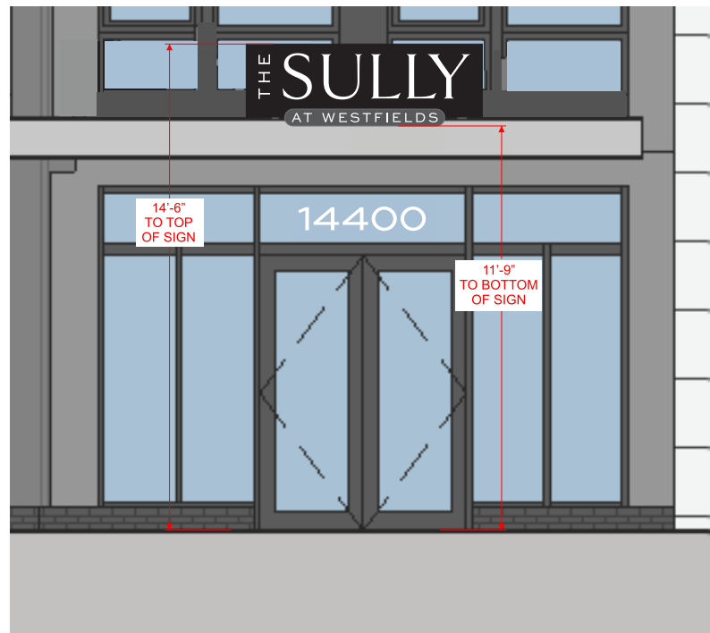
A401:2A NORTH ELEVATION (PARTIAL) 1" = 5'
