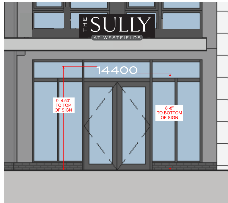
A401:2A NORTH ELEVATION (PARTIAL) 1" = 5'
