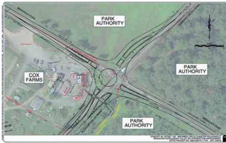
VDOT's diagram of the proposed roundabout at Braddock and Pleasant Valley roads in Centreville.
